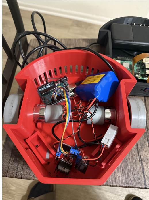
Figure 5: Bottom Level wiring, Before mounting of Arduino and Battery
